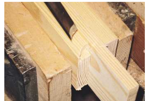
▲ Pic.18 ...produces the correctly shaped rebate for the moulding on the stiles
